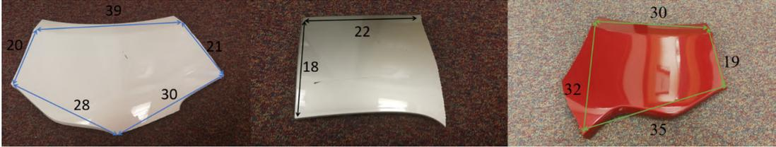
Fig. 2.7 Automotive bumpers with solid paint, metallic paint and pearlescent paint used for the experiments.
