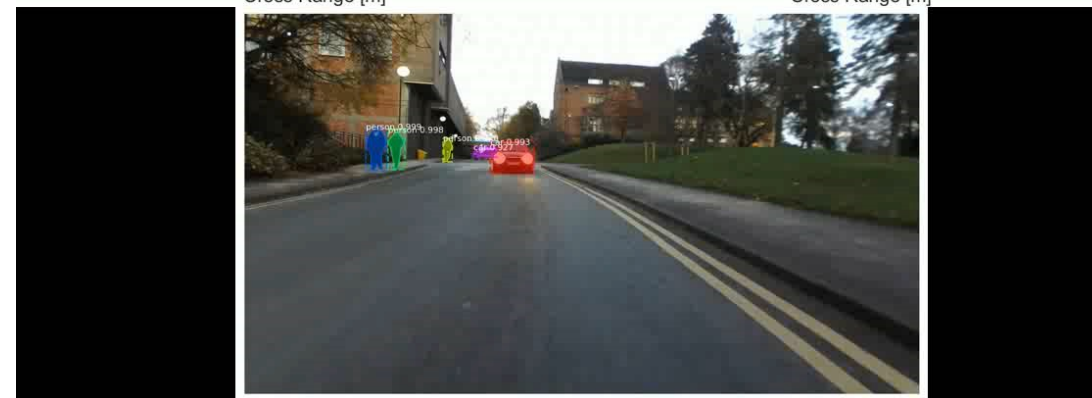
Segmented optical imagery using Mask-RCNN
